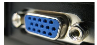
This is a standard VGA connection. This is totally fine!
